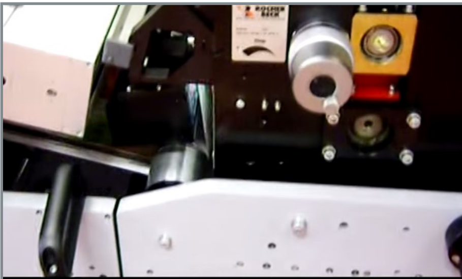
CC1 camera monitoring and correcting for register errors
