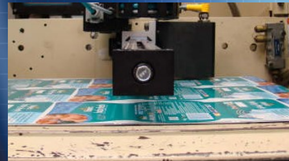
CC1 camera monitoring and correcting for register errors
